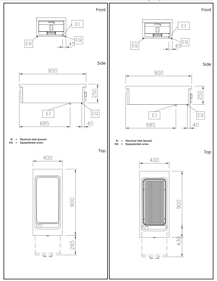
Modular Cooking Range Line thermaline 90 - Half Module Electric Fry Top, 1 Side-Marine
